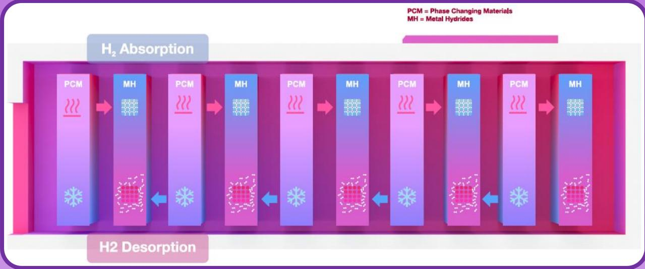
The tank is based on an innovative concept that couples hydrogen and heat storage for stationary storage of the excess renewable energy.
