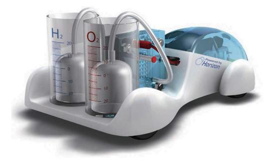
The Hydrocar uses a reversible fuel cell with a proton exchange membrane (PEM). Generates electricity by consuming hydrogen located in the onboard hydrogen storage cylinder which reacts with oxygen, which is also created and stored on board the kit.
